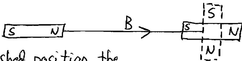
If  $M_2$  were in the dashed position, the torque would take it to the solid position. so  $\alpha_2 = \phi$  so yes it makes sense
