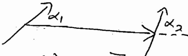
$$V = \frac{\mu_0}{4\pi R^3} \left[ \vec{m}_1 \cdot \vec{m}_2 - 3(\vec{m}_1 \cdot \hat{R})(\vec{m}_2 \cdot \hat{R}) \right] \quad \alpha_1 \text{ is fixed}$$
