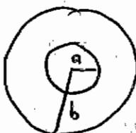
$U = \frac{1}{2} L I^2 \quad U = \int_{\text{all space}} B^2 / 2\mu_0 dT \quad B \text{ is only nonzero between } a \text{ and } b$
